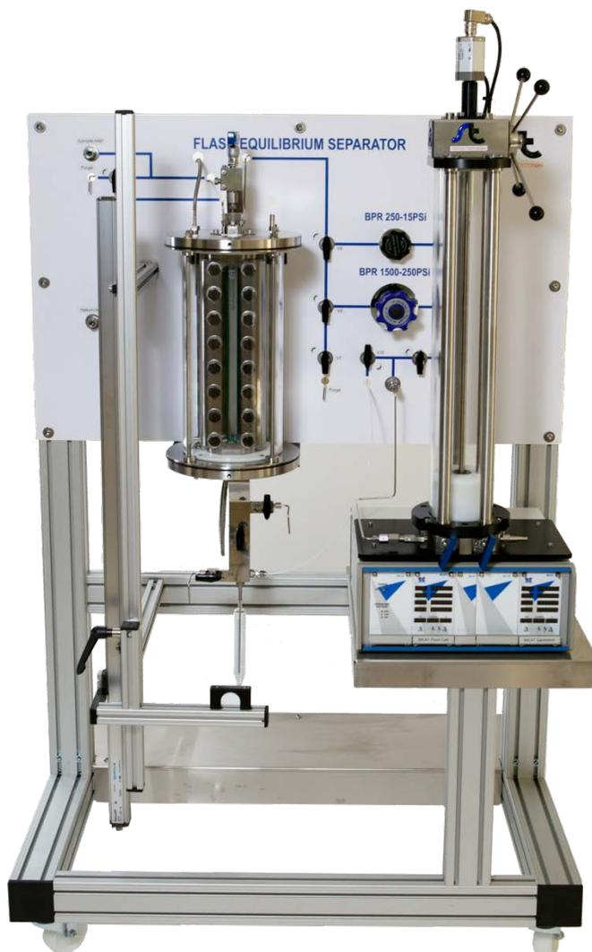
Our Flash Equilibrium Separator is dedicated to the study of gas expansion of oil samples under pressure with the aim to optimize the separation of the oil/gas phase and the gas/oil ratio.
