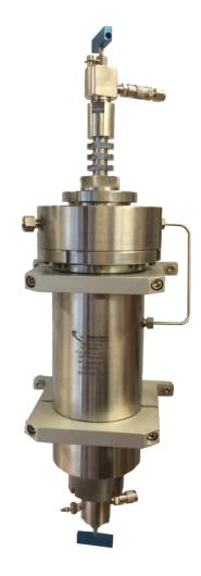
ST hydrostatic or also called biaxial, core holders are standard type core holder defined by having common radial and axial pressure. In general, these core holders are dedicated to gas and liquid permeability flooding and aging experimentations. The sample is inserted through the loading end and an adjustable floating piston ensures the solid maintain of the sample of any length.
