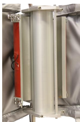
The Heating Jacket
