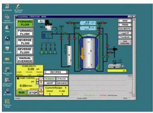
monitoring the change in permeability as fluids invade deeper into the core as well as the determination of skin factors which may influence the testing results.
